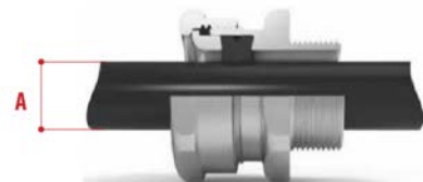
Cable gland with gasket with unarmored cable
